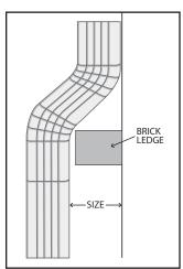
We have several varieties of offset downspout connections to transition gracefully over a brick ledge. You can eliminate the awkward look of a two-piece configuration with our choice of 1" to 6" away-fromthe-wall options.
