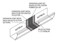
A 50' section of gutter can potentially expand almost 2/3 of an inch from winter to summer causing gutters to buckle. Expansion joints are a preventive measure for excessive movement in the gutter, and should be mounted in place every 50' of exceptionally long gutter runs.
